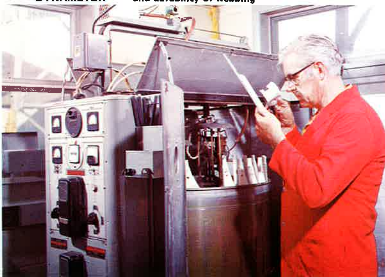
WEATHEROMETER: INSTANT YEAR ROUND CLIMATIC CONDITIONS
