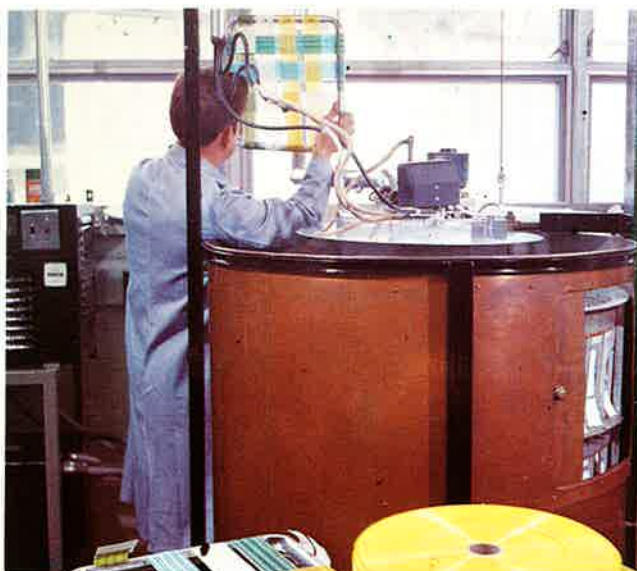
ACCELERATED TESTING UNIT: for fading, color stability via ultra-violet rays, dampness, wetness
