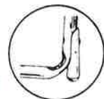
NON-TIP LEG CONSTRUCTION ON FRONT LEG OF ARM CHAIR
