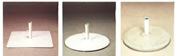
#12 Steel Market Base Pattern #1 Pebble, #3 Green, #5 White and #7 Antique Black, 55lb, 10" stem, 24" square. #17 Cast Iron Market Base Pattern #1 Pebble, #3 Green, #5 White and #7 Antique Black, 66lb, 10" stem, 24" diameter. #21 Pre-Cast Market Base Pattern #5 Off-White
