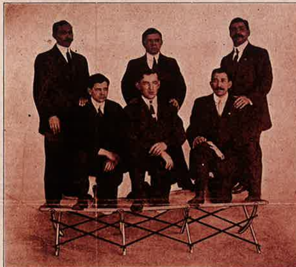
An actual photograph showing the Telescope Cot Bed sustaining a weight of 940 pounds.
